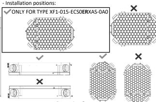
The Xflat unit must be installed and put into operation in accordance with the general and locally valid safety regulations, by a person with adequate education, experience and knowledge of the relevant regulations, standards and possible risks and possible dangers, or by a suitably trained service technician. Failure to follow the installation procedure may result in damage to the unit, malfunction, and possible injury to the user's health and property.
